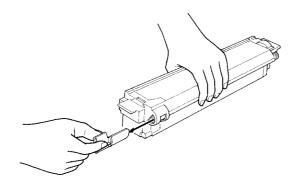
6. Slide the new toner cassette into the machine along the rails until it stops.
